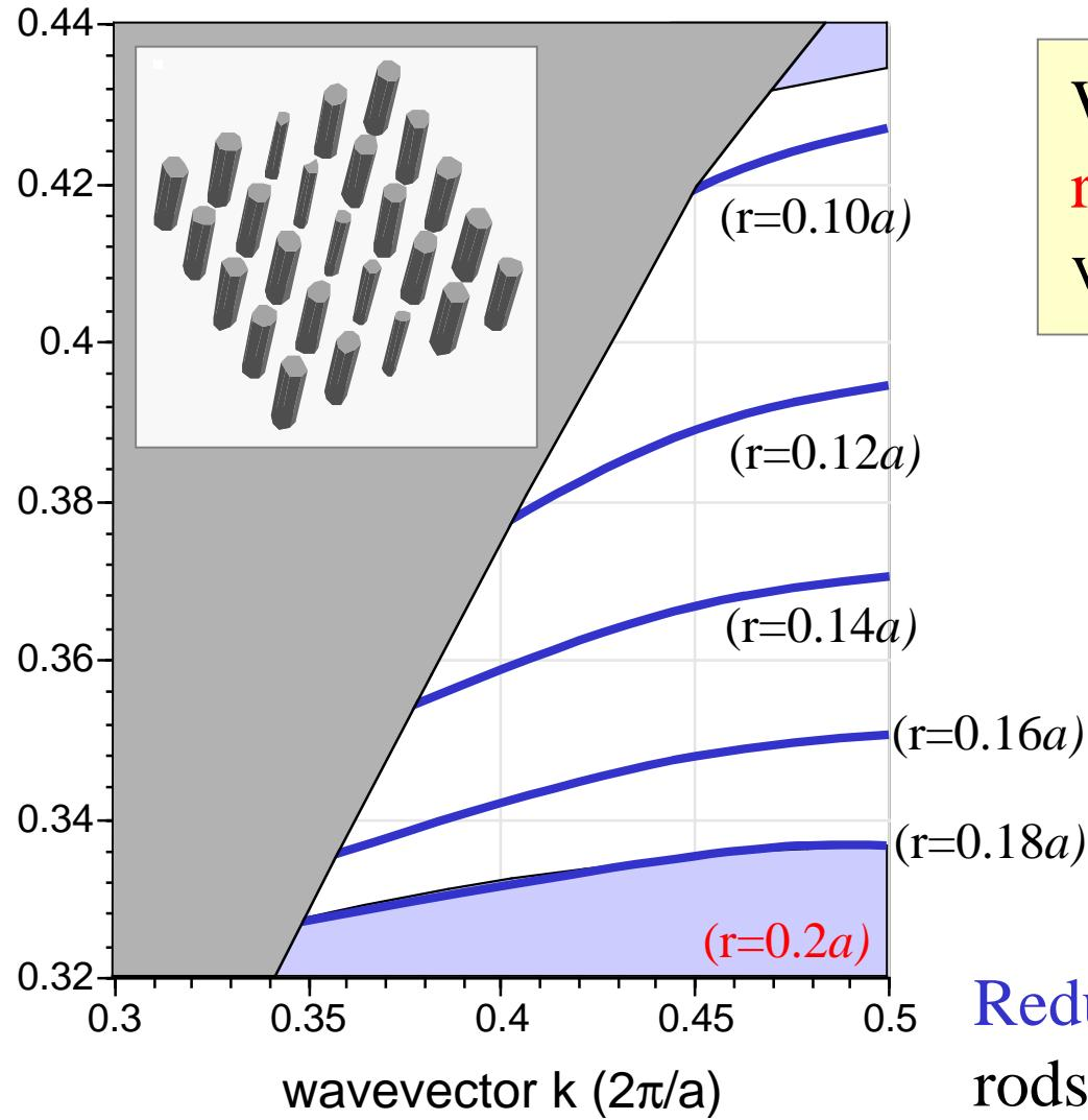
We *cannot* completely remove the rods—no vertical confinement!
