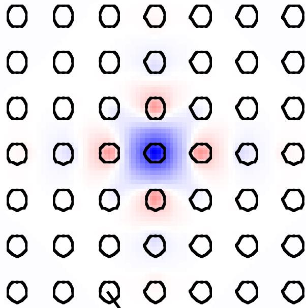
Lower the  $\epsilon$  of a single rod: push up a monopole (singlet) state.
